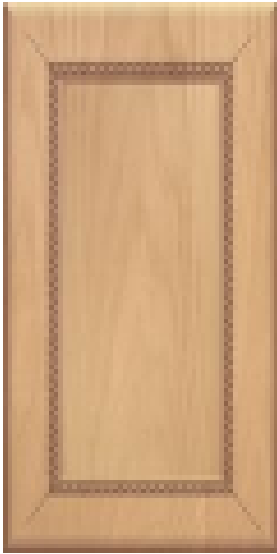
Mitered Square, Flat Panel Style #02 3/4" Thick Mitered Construction with 3/8" Solid Flat Center Panel and rope moulding trim on panel
