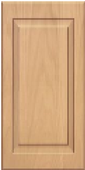
Mortise & Tenon, Raised Panel Style #15 3/4" Thick, MDF core door. White satin ThermalFoil covered
