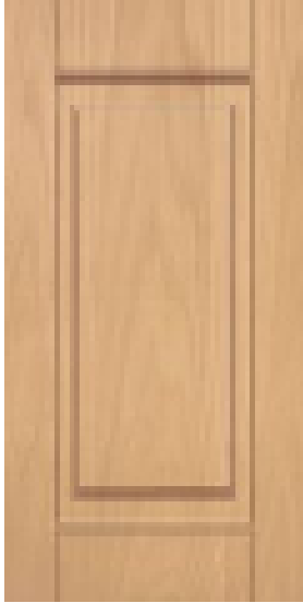
Mortise & Tenon, Raised Panel Style #03 3/4" Thick Mortise & Tenon Construction with stairstep detail on interior of rails only and 5/8" Thick Square Raised Center Panel
