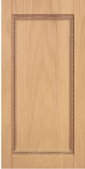
Mortise & Tenon, Flat Panel Style #03 3/4" Thick Mortise & Tenon Construction with 1/4" Flat Veneer Center Panel and rope moulding trim on panel
