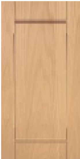
Mortise & Tenon, Flat Panel Style #10 3/4" Thick Mortise & Tenon Construction with 1/4" Flat Veneer Center Panel
