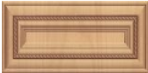
Mitered Drawer #15 3/4" Thick Mitered Construction with 3/8" flat veneer center panel and rope moulding trim on panel
