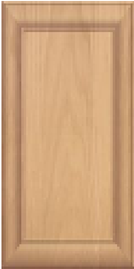
Mitered Square, Flat Panel Style #03 3/4" Thick Mitered Corner Construction with 1/4" radius corners and 3/8" Solid Flat Center Panel
